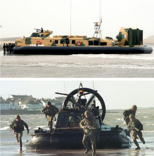
A hovercraft's skirt means that it requires much less lift power than would be expected, while still giving the vehicle many of the benefits of flying. Requiring less power means that fuel consumption is drastically lower, while also allowing for much more payload to be carried than any competing air vehicle.
